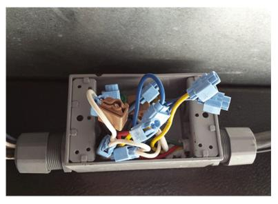
**4.** Aftermarket trailer sway control devices, like the example shown below. These devices can apply the trailer's brakes to control trailer sway. When this happens, the truck will detect this and set DTC C1114. It will also display a "Service Trailer Brake" message on the DIC.
