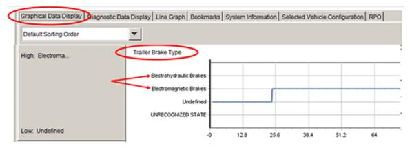
To view "Trailer Brake Control Output Circuit" 47 faults, build GDS2 as follows: CCM->Data Display -> parameter "Trailer Brake Control Output Circuit": Okay, Short to Ground, Short to Power, or Unknown. Example, shown below is a trailer with a short to ground on the trailer brake circuit.
