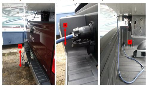
3. Poor trailer wiring connections, as shown below. General Motors does not recommend these type of connections, but many trailers utilize these connections. These type of connections are not robust and are not recommended, especially for brake wiring.
