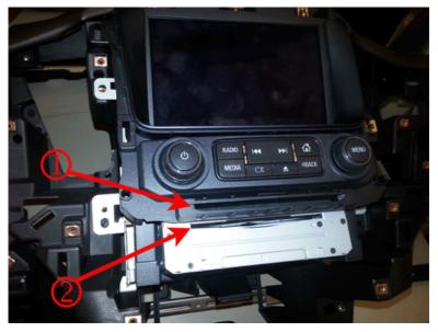
The ICS and multimedia player use two common locating pins (3), as shown below. When the ICS is installed, the two common locating pins (3) may not properly engage into the holes in the back of the ICS, causing the condition.
