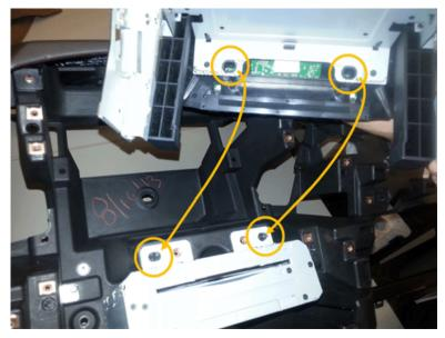
After reinstalling the ICS and multimedia player make sure the slots are aligned, as shown.
