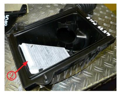
If the Hydro Carbon Absorber is missing, or the ID code is other than ACD, replace the Air Cleaner Housing with the latest listing in the Electronic Parts Catalog If the Hydro Carbon Absorber is present and the ID code is ACD, refer back to current SI diagnostics.
