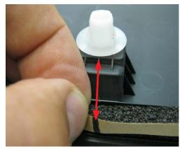
7. CAREFULLY peel the backing and working SLOWLY outward from the center point, start to apply the EPDM foam INSIDE the molded lip along the back edge of the scoop. While being careful not to stretch the foam while applying it, work the foam around the previously installed protectors as shown in the photos below.
