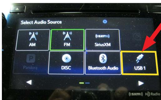
Install Drive “1” (or Drive “2” after successful installation of Drive “1” update is confirmed) into the vehicle’s USB port. After the flash drive is recognized, the USB icon will illuminate.
