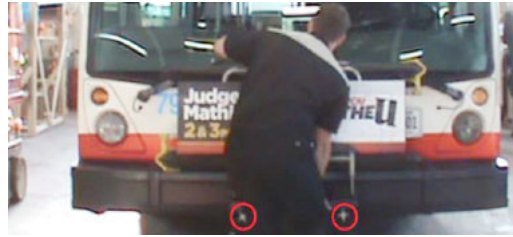
Figure 51 - Install the Bicycle Rack
