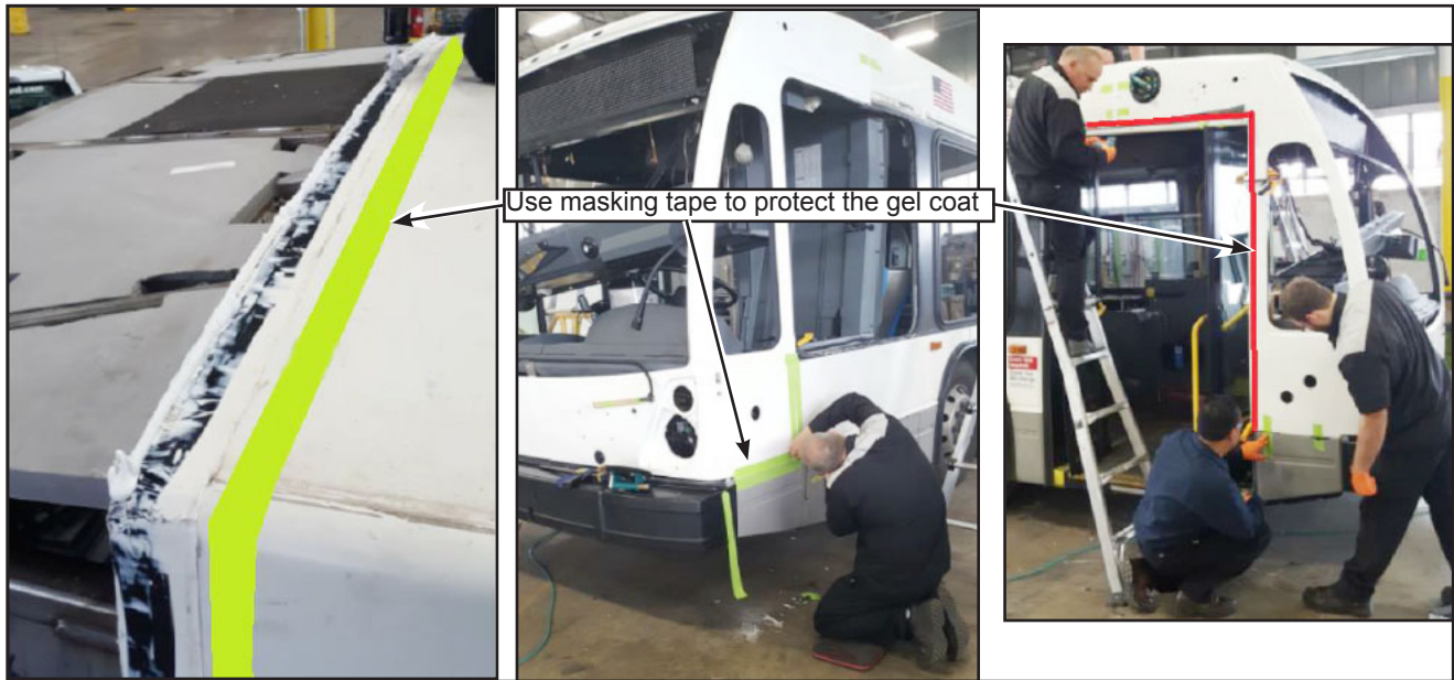
Figure 27 - Protect GelCoat with Masking Tape
