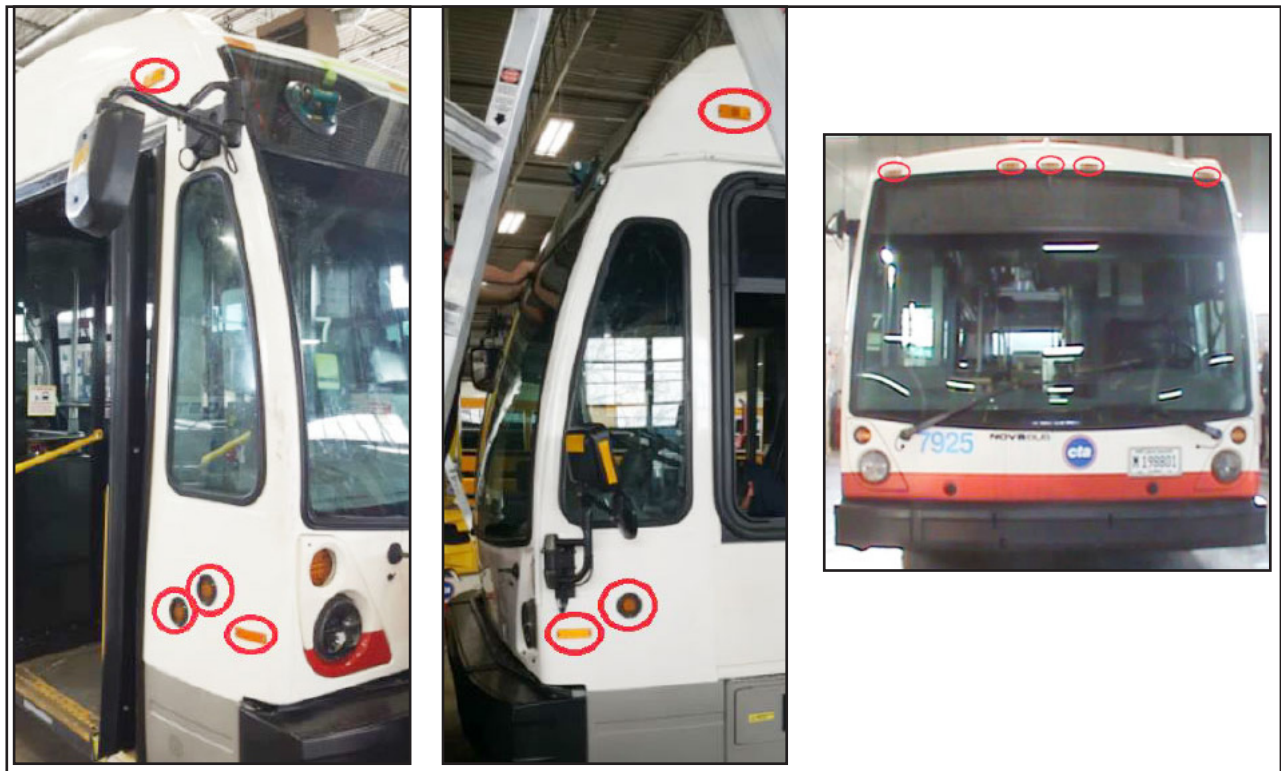
Figure 47 - Install Reflectors, Marker Lights and Signal Lights
