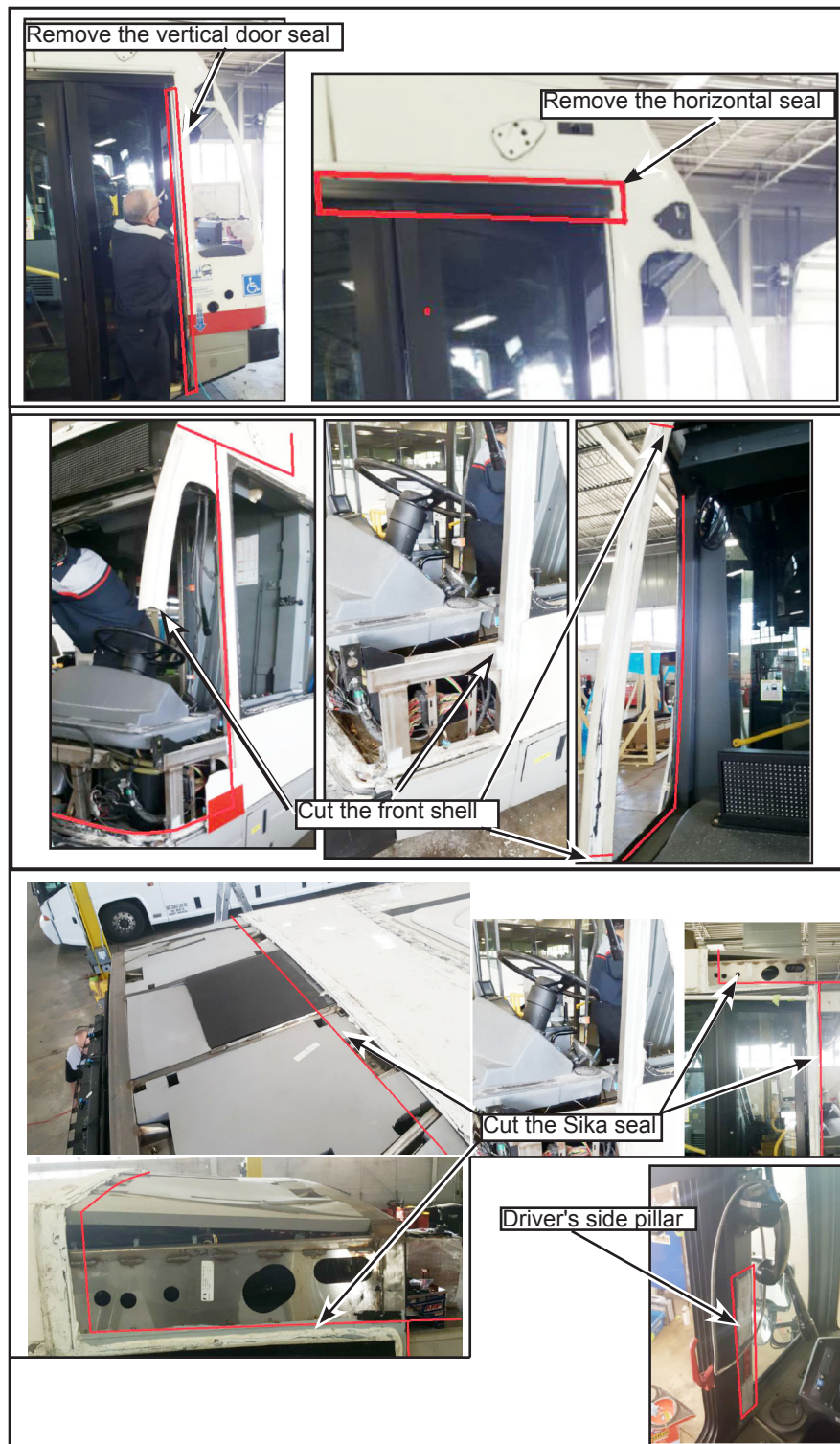
Figure 21 - Remove the Front Shell
