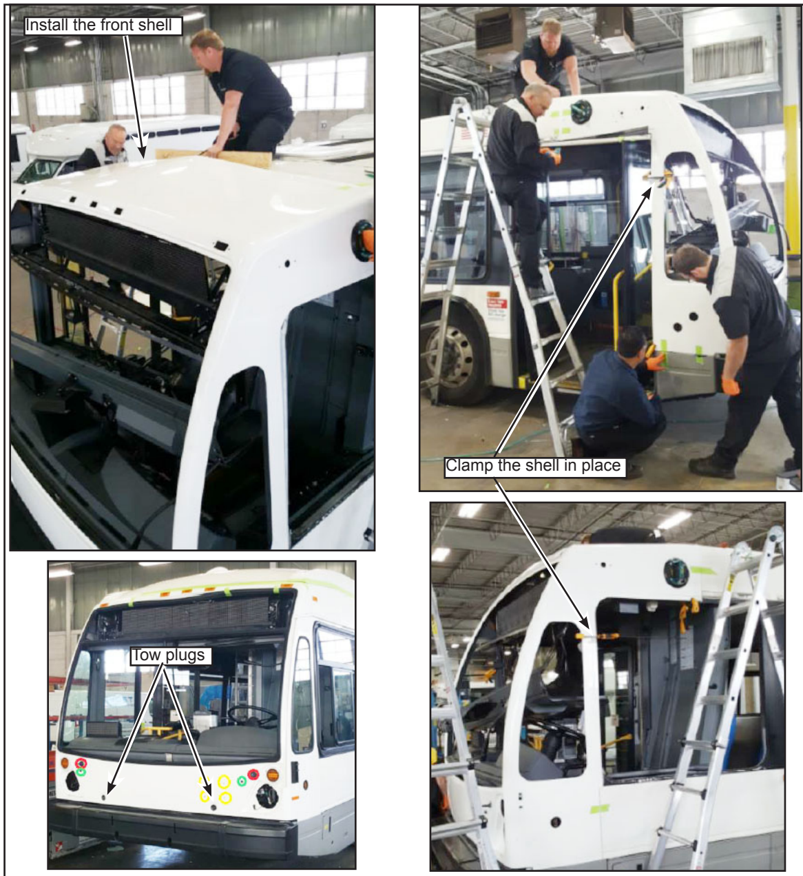
Figure 29 - Install the Front Shell
