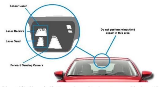
If the windshield is repaired in this area, it may affect the performance of the Forward Sensing Camera and/or Laser Sensor. This may cause incorrect detection of objects and improper operation of i-ACTIVESENSE system(s).
