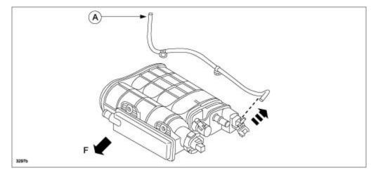
b. Install the Canister Hose (PE01-13-971) (B) to the Charcoal Canister outlet.
