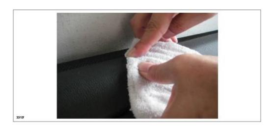
**NOTE:** Press the trim around the dent with your fingers and rub toward the center of the dent (as shown by the arrowsbelow).
