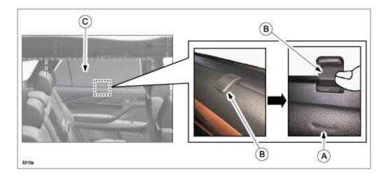
A cushioning material (A) has been attached to the backside of tab, so the tab will no longer directly contact the trim.
