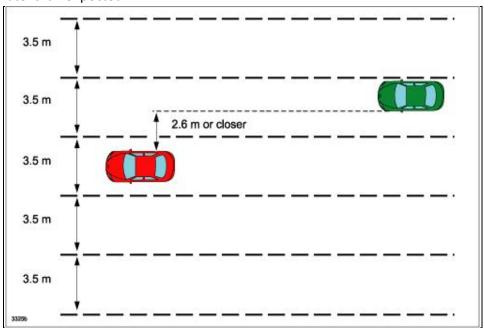
3. BSM indicator light on the outer mirror glass illuminates even when a vehicle is approaching two lanes away (right or left side).
