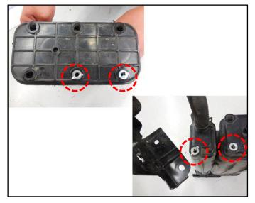
8. Inspect for any cracks at the canister insert nut surfaces or in the surrounding plastic at the bottom and top of the canister.
