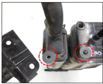
Tightening Torque 4.9 ~ 5.9 Nm (0.5 ~ 0.6 kgf.m, 3.6 ~ 4.3 lb-ft)
