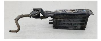
Remove the 6 mounting bolts from the canister lower and upper brackets.
