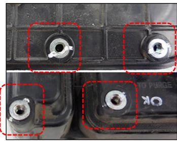
Examples of cracks found at the insert nut (C) or in the surrounding plastic.
