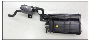
3. Remove the mounting bolts from the canister's lower and upper brackets. **Veloster** has 4 bolts total to remove.
