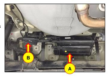
Canister, filter and brackets shown removed as a complete assembly from the vehicle.
