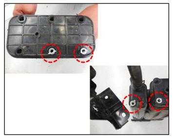
6. Inspect for any crack(s) found at the canister insert nut surfaces or in the surrounding plastic at the bottom and top of the canister.
