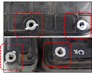
Examples of cracks found at the insert nut (C) or in the surrounding plastic.
