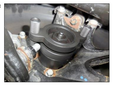
12. Tighten the 32mm assembly nut using a socket wrench.
