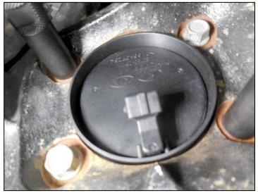
29. Check that the WSS cover is correctly installed by verifying that the cover is underflush (deeper) compared with the knuckle surface level.
