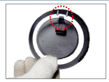
20. Insert the installer/WSS cover into the SST assembly with the WSS cover connector aligned with the hole in the SST.
