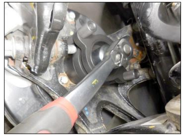
15. Remove the support nuts by hand.
