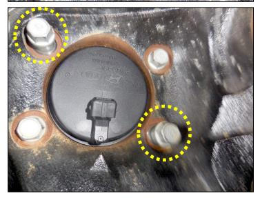
Reinstall remaining parts in reverse order of removal. 31. Repeat the wheel speed sensor cover replacement for the other side of the vehicle. Check and clear any DTCs. Verify no warning lamps on in the instrument cluster.
