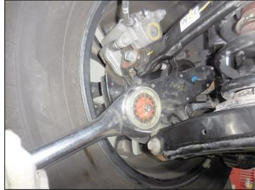
27. Remove the support nuts by hand and remove the SST assembly.
