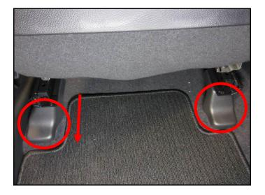
5. Remove the four seat bolts using a 14mm socket and ratchet.
