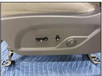
9. Remove the Phillips screw located on the left side of the seat, and pull the cover to the left as shown in the picture.
