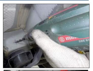
13. Remove the 6 plugs along the frame rails
