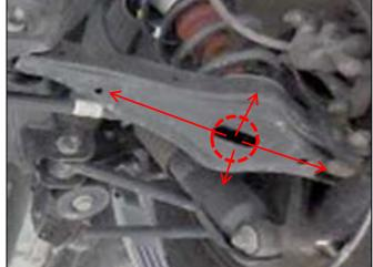
1. Front cross member – Interior surfaces (using "inside" nozzle)
