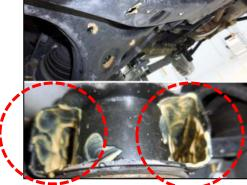
2. Front lower control arms – Interior surfaces (using "*inside*" nozzle)
