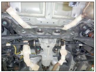
8. Locate the areas A and B near the front cross member mounting bolts.
