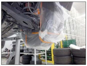
7. Wrap the exhaust areas adjacent to the front and rear cross members with plastic bags to protect them from overspray. Use tape to secure the plastic in place.
