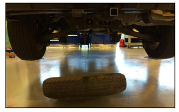
2. Open the vehicle's tail gate, remove the cover for the bolt to lower the spare wheel/tire assembly, and loosen the bolt to lower the spare.
