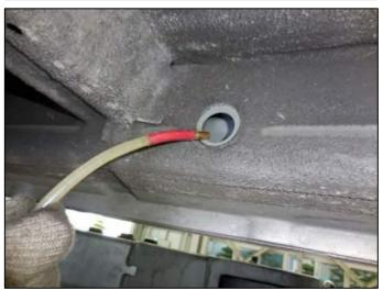
3b. Insert a plug into each hole after spraying the cavity wax.
