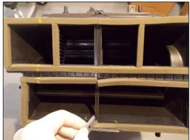
Using a putty knife or a gasket scraper, carefully loosen the white insulation pad from one side of the Heater & Evaporator Assembly to expose the joint between the 2 case halves.
