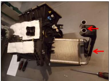
3. Remove the (8) screws from the plastic cover over the A/C evaporator using a Philips screwdriver, and then remove the plastic cover and the A/C evaporator.
