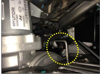
10b. Some wire harness anchors must be disengaged to allow MDPS assembly to be released.
