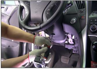
5a. On some models, it is required to turn the steering wheel left/right 90 degrees to access the shroud mounting screws.
