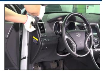
2. Use a plastic trim tool to remove the crash pad side cover (A).
