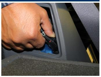
This photo shows the 12V service connector disconnected from the vehicle.
