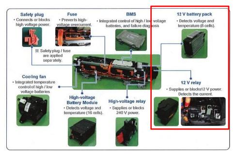
The 12V integrated LiPO battery system has automatic severe discharge protection. When battery discharge occurs down to 10% SOC, a 12V power relay deactivates electrical power to the vehicle. The vehicle will not have power door locks, interior lights, and the dash will not illuminate.
