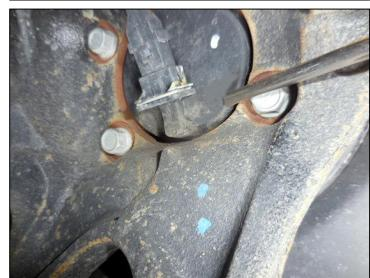
4. Spray silicone on the wheel speed sensor connector body that protrudes from the bottom of the WSS cover.
