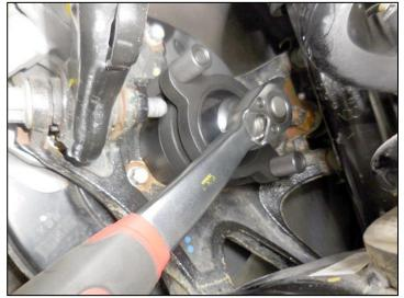
15. Remove the support nuts by hand.
