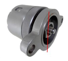
10. Insert the SST assembly onto the support bolts, and press inwards tightly until a sticking sound is heard.
