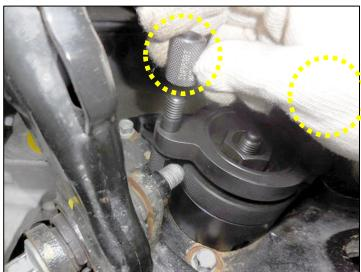
16. Remove the SST assembly by pulling it off. The WSS cover should come with the tool inside the collet.
