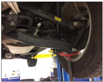
Remove the WSS plug by pressing the spring clip and pulling the plug upwards 3. off the connector.
