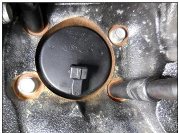
30. Remove the support nuts, and install the previously removed hub bolts.
