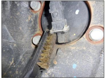
3. Wipe the connector area clean with a cloth, and use compressed air and an air nozzle to blow out any remaining debris.
