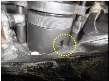
24. Install the support nuts onto the support bolts in the orientation shown by the yellow arrows below.
