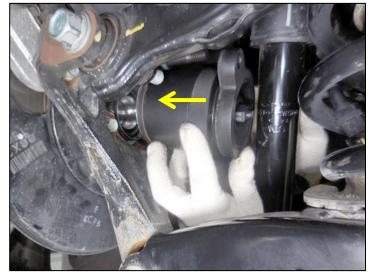
23. Rotate the tool until the inspection hole is aligned with the mark on the bottom of the knuckle.
