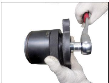
18. While holding the WSS cover, tap the collet stud using a rubber mallet from the opposite side to loosen the collet from the SST assembly.
