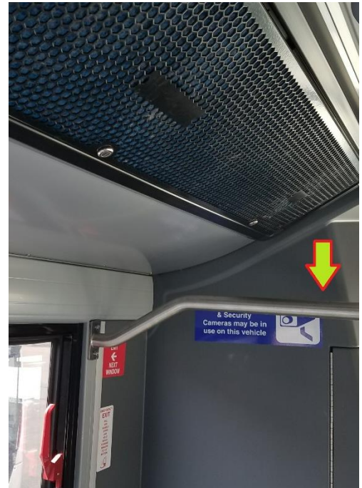
Figure 2: Stanchion to be removed
