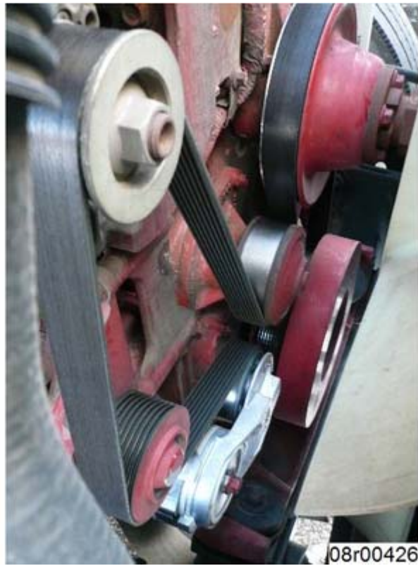
Figure 1, Fan Drive Belt Configuration with Cummins Supplied Fan Drive Installed.
