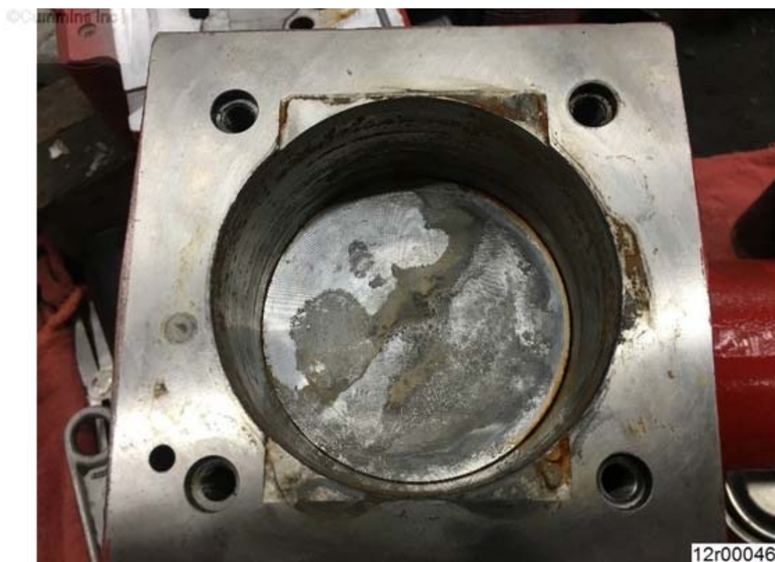
Figure 4, Corrosion Present in Air Compressor Cylinder.
