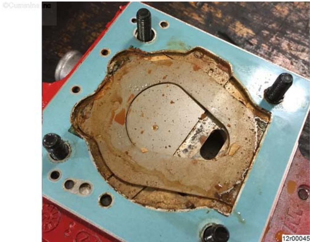
Figure 3, Corrosion Present On Air Compressor Unloader and Valve Assembly.
