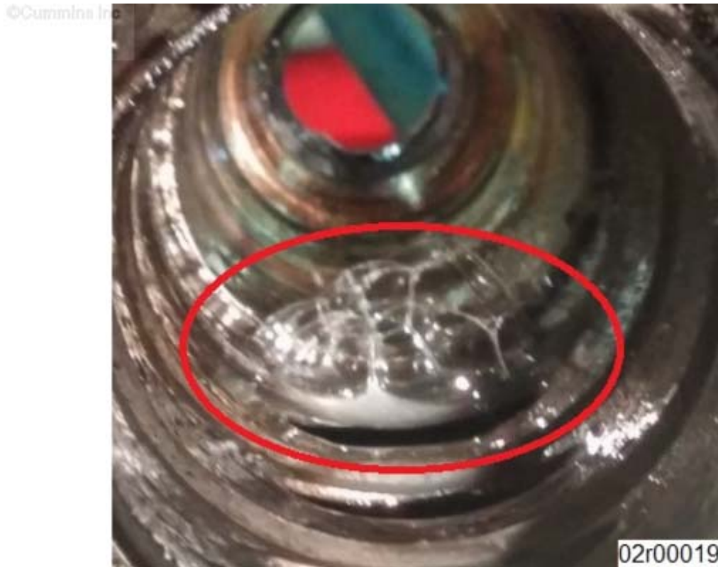
Figure 2, Large Amount of Coolant Leakage Past Injector Sleeve.
