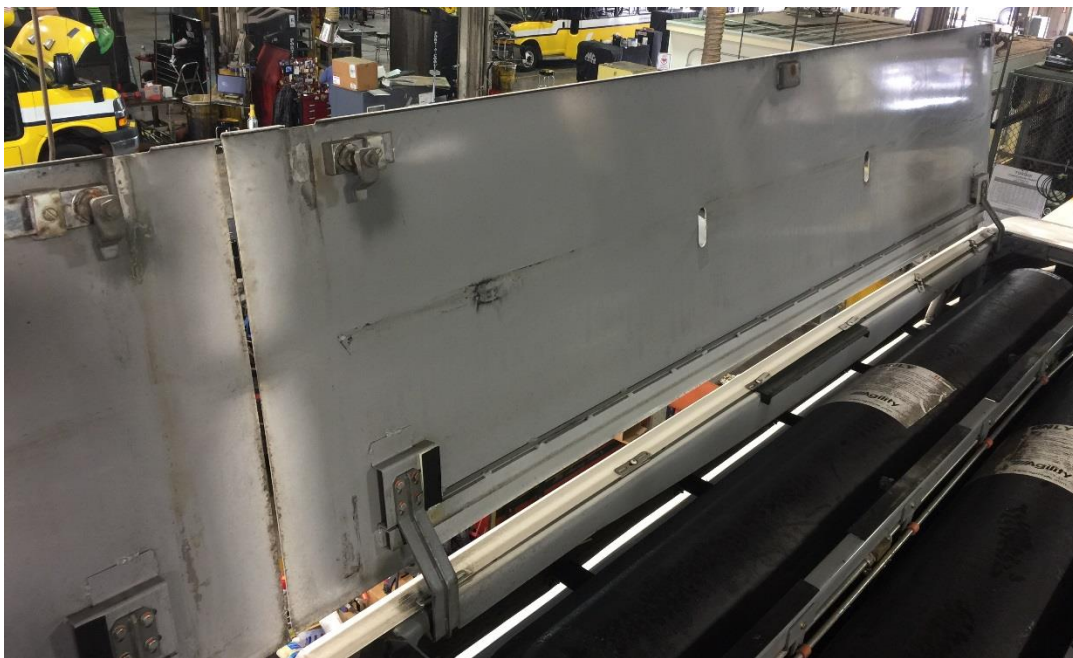
Figure 6 In most cases, scuff marks or dirt can provide a perfect guide for the placement of new rubber strips on the doors.
