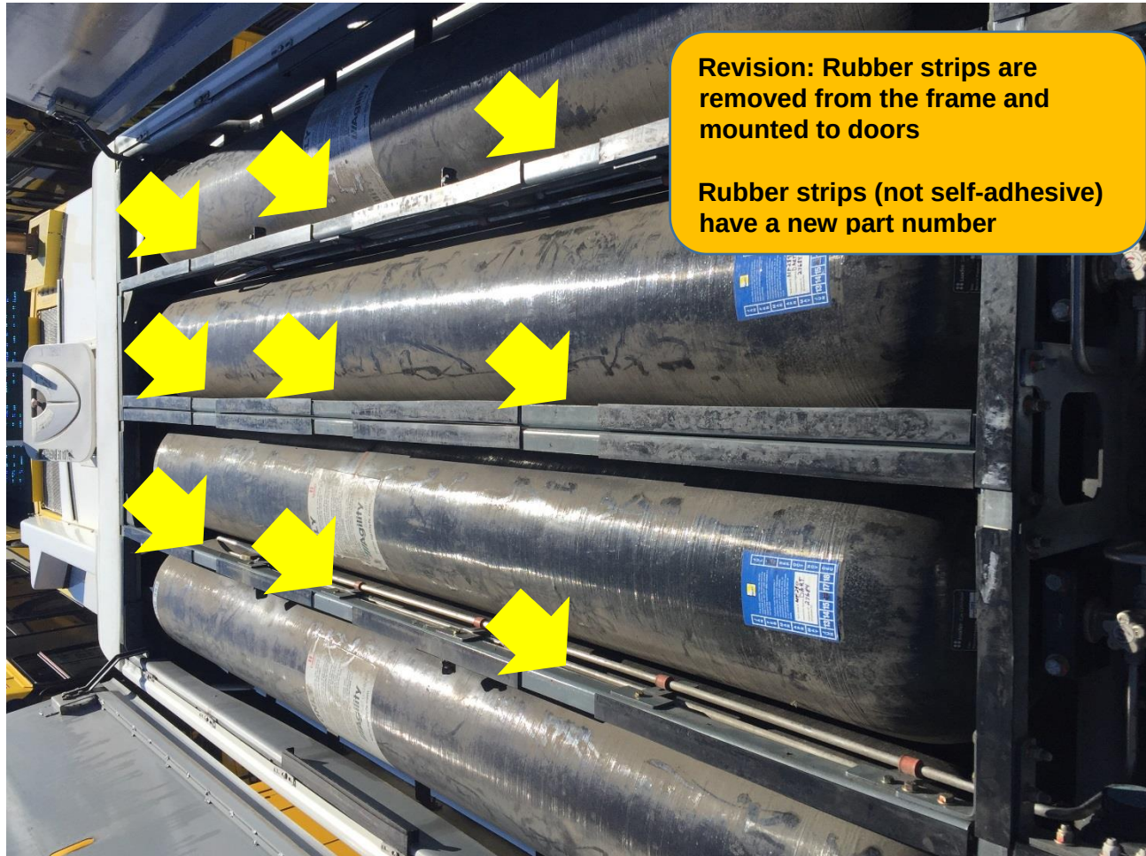
Figure 1 FOR REFERENCE ONLY. Rubber isolators on roof mount systems are to be replaced with new 3M tape and rubber strips on the mating surfaces on the doors. Surface preparation is important for proper adhesion.
