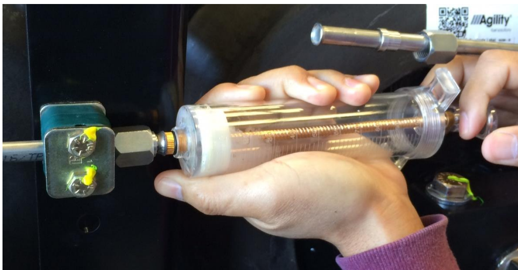
Figure 7 Draw the water out, using suction from the syringe.
