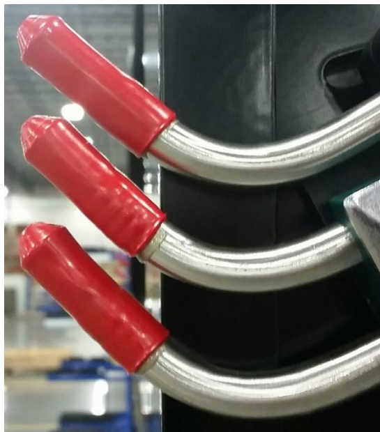
Figure 10 Correctly installed vent caps.
