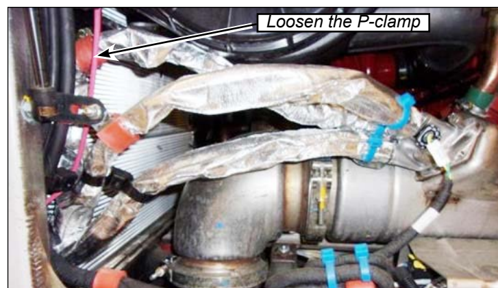
Figure 8 - Loosen the P-Clamp on the Upper Coolant Line
