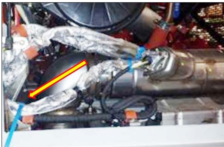
Figure 11 - Reposition the Lower Coolant Line
