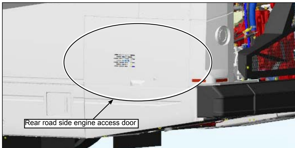
Figure 2 - Open the Rear Road Side Engine Access Door
