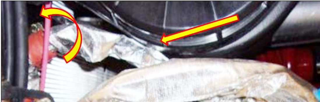
Figure 9 - Position the Upper Coolant Line
