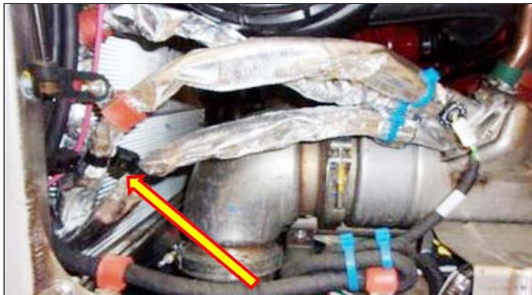
Figure 10 - Remove the Tie Wrap
