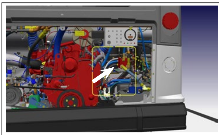
Figure 1 - Location of the Hydraulic Fan Control Manifold
