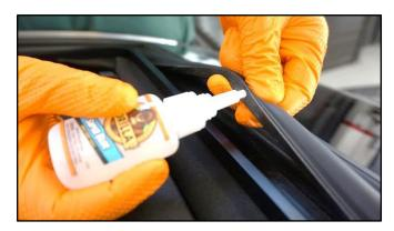
Push the weather strip down onto the sunroof frame and apply pressure for approximately 30 seconds until the weather strip has properly adhered to the sunroof frame.
