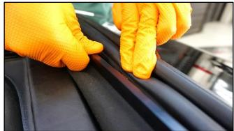
5. After ensuring that the adhesive has cured, open and close the sunroof several times to confirm proper installation of the weather strip.
