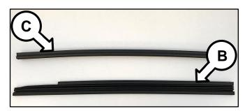
3. Reinstall in the sliding bracket to the upper sliding rail (C) without the folding cover (B) attached. Ensure the sliding bracket is completely secured at all four (4) locations shown.
