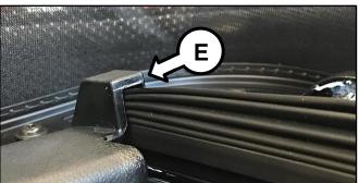
6. Ensure complete attachment of the bottom of the folding cover to the lower sliding rail.
