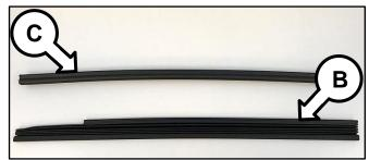
Reinstall in the sliding bracket to the upper sliding rail (C) without the folding cover (B) attached. Ensure the sliding bracket is completely secured at all four (4) locations shown.
