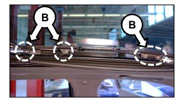
4. With the assistance of another person, remove the panoramic sunroof glass by sliding the glass towards the front of the vehicle until the sliders are out of the tracks (C).
