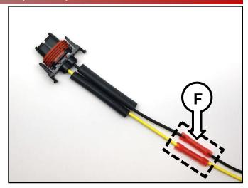
Crimp the butt splice connectors at two
