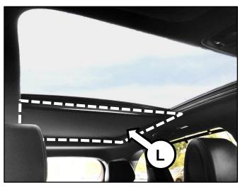
9. Gently and carefully pull down the headliner (M) at the right front corner, approximately two (2) inches to access the roller guide retaining screws.
