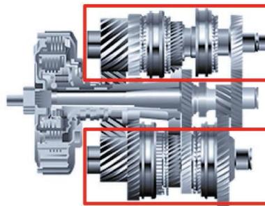
Gear set 2 (controlled even gears)
