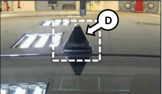
6. Install the new antenna. Reinstall all removed components in the reverse order of removal.
