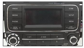
Press and hold preset button "1" and then preset button "4" and continue to hold both for five (5) seconds.
