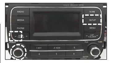
14. Once the update is complete, the screen as shown will be displayed (Update Complete). Press the power button to restart the unit.
