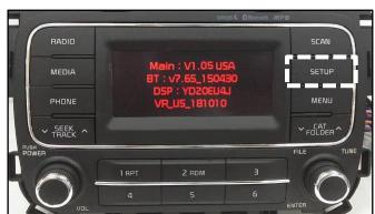
10. Press preset button "1" to display the firmware upgrade menu.
