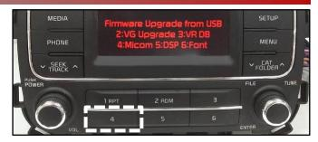
12. In some cases, the firmware upgrade (1/2) will begin and system will display the progress on the screen. Once the upgrade is complete, the head unit will automatically reset and then turn off. Monitor this part of the upgrade to ensure the second upgrade begins (see step 13 below).
