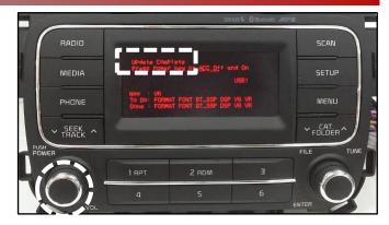
15. Verify that the software upgrade is successful by checking the software version by following software inspection procedure steps 3 to 6 on page 2 of this bulletin. If update is not successful, restart the procedure from step 3.
