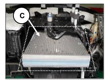
6. Replace the evaporator core with a new one.
