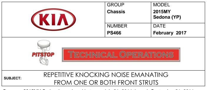
On some 2015MY Sedona's produced between July 21, 2014 through September 21, 2014, customers may complain of a repetitive knocking noise emanating from the front strut or suspension areas of the vehicle. This noise is more noticeable during a parking lot maneuver at slow speeds, especially over speed bumps.
