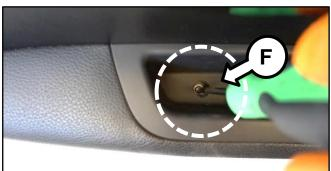
7. Remove the door panel. Leave the 2 master switch harnesses connected to allow for glass retaining bolt alignment in step 9.
