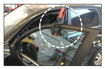
12. Remove the handle trim cap bolt cover and loosen the outside door handle trim cap bolt (K).
