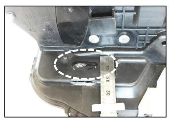
4. Insert the clip with the flat side into the slot as shown.
