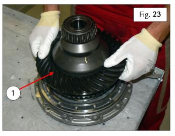
Fit the differential crown wheel (1) onto the differential cover – Fig. 23.
