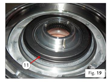
Install the spring ring (11) on the "Z" ring - Fig. 19.
