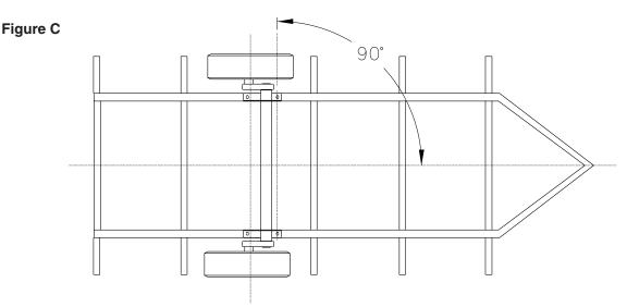
To ensure proper tracking, the axle must be placed on the frame perpendicular to the centerline of the vehicle. The accuracy must be within plus or minus one half degree. For multiple axle applications, each axle must be parallel with the others within one sixteenth of an inch when measured at the wheel centers.
