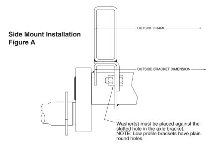
Side mount hangers should be welded to frame with three (3) <sup>1</sup>/<sub>4</sub>" fillet welds, 2<sup>1</sup>/<sub>2</sub>" long on each side of the hanger and a fillet weld on each end. Welds should meet the quality standards of the American Welding Society, D1.1, Structural Welding Code.
