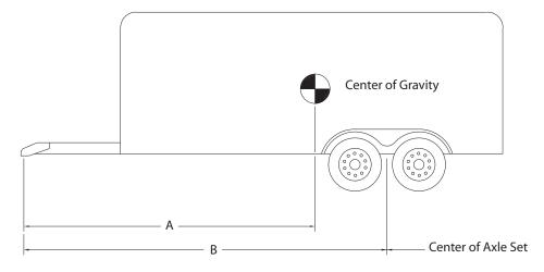
Note: "Center of Axle" on a Torflex® axle is defined as the center of spindle.
