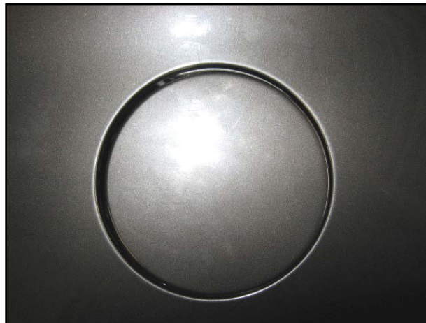
Figure 1 - Fuel Filler Door Not Aligned
