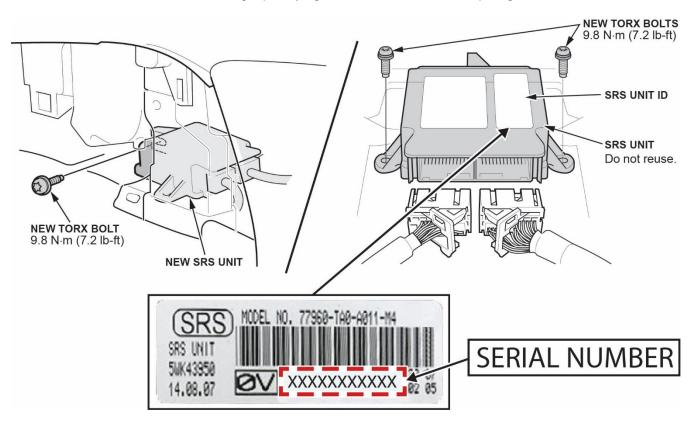
8. Connect the SRS connectors to the SRS unit by pushing the connector in and the lever moves to the locked position.
