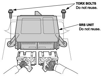
7. Write down the new SRS unit ID (serial number) on the RO, then install the new SRS unit using the new Torx bolts. NOTE: Make sure the SRS unit is sitting squarely against its bracket before torqueing the Torx bolts.
