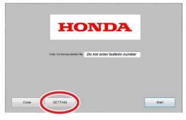
1. Update the PGM-FI or A/T software by selecting the i-HDS Diagnostic System icon. Refer to Service Bulletin 01-023, *Updating Control Units/ Modules*.
