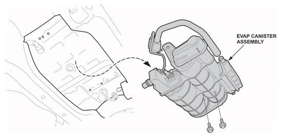
4. Check for a protector on the purge tube. If the vehicle does not have a protector, install one as shown. Otherwise, go to step 5.
