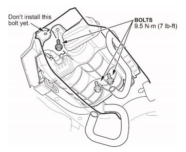
13. Install the filter onto the bracket and secure it with the bolt.
