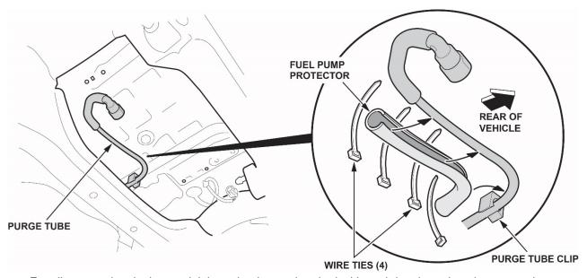
• Equally space the zip ties, and tighten the ties so that the locking tab is oriented on the top as shown.
