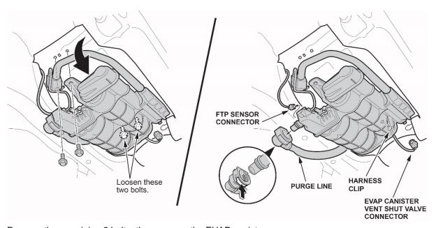
3. Remove the remaining 2 bolts, then remove the EVAP canister.
