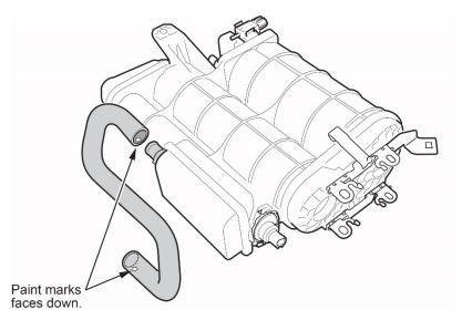
8. Install the new canister drain kit (includes drain box, hose, and clip) but do not connect the other end of the hose at this time.
