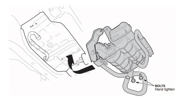
11. Connect the purge lines, the EVAP canister vent shut valve connector, and the FTP sensor connector.
