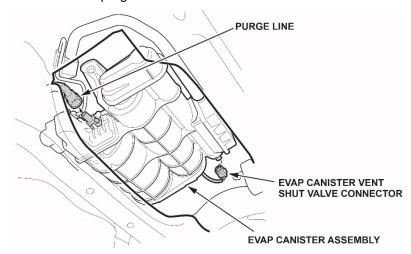
2. Loosen the two bolts on one side of the canister and remove the other two bolts as shown, then disconnect the second purge line, FTP sensor connector, and the EVAP canister vent shut valve harness clip.
