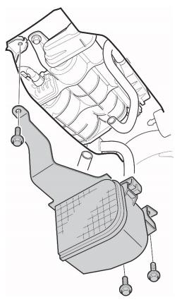
3. Remove the bolt securing the canister filter box to the bracket, then remove the canister filter box.
