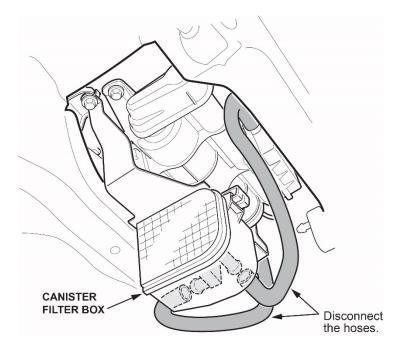
2. Remove the three bolts as shown and remove the canister filter box and bracket from the vehicle.
