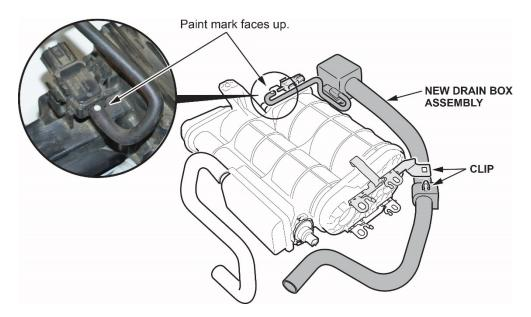
9. Install the new drain box bracket (non-hybrid only) and the new retainer as shown.
