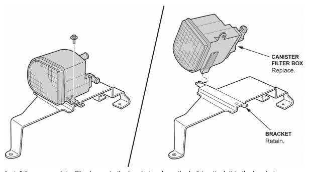
4. Install the new canister filter box onto the bracket and use the bolt to attach it to the bracket.
