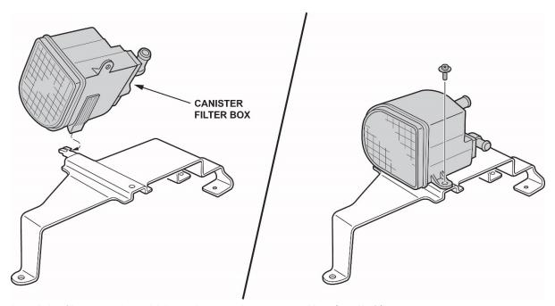
14. Install the filter onto the vehicle and torque the nut to 12 N-m (6.9 lb-ft).
