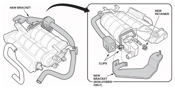
10. Install the EVAP canister assembly with the bolts shown finger tight.
