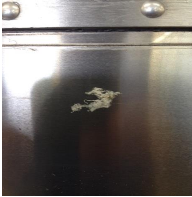
Picture of Filiform Corrosion
