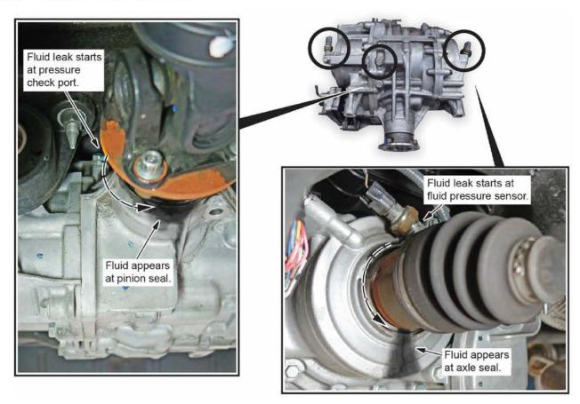
Before considering rear differential replacement, be sure to check those items carefully. The repair could be as easy as tightening/replacing the fluid pressure sensor or tightening the fluid pressure check port.
