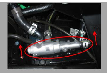
4. Verify there is adequate (3/8" or more) clearance between the hose and the shear plate.
