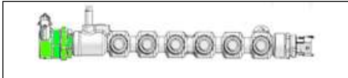
Figure 3 Fuel Rail Pressure (FRP) Reduction Valve on Fuel Rail
