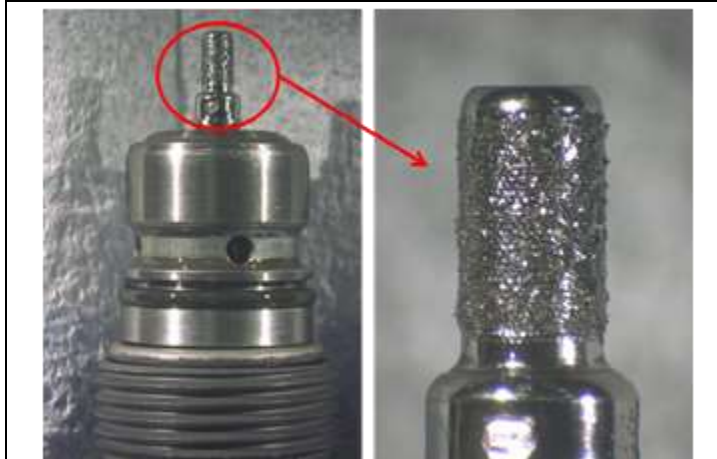
Figure 4 FRP Reduction Valve with magnetic debris (part is bad)
