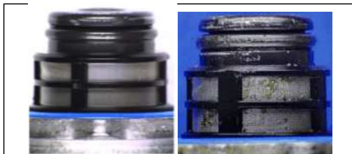
Figure 2 Fuel Pressure Regulator with and without magnetic debris (Good part on left) (Bad part on right)
