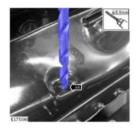
11. Using a suitable larger drill, deburr by hand both sides of the drilled holes.
