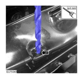
Using a suitable 5.5mm drill, drill the four (4) suspension mat fixation holes.
