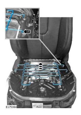
Using a suitable 4mm drill, drill a pilot hole to the four (4) suspension mat fixation holes.
