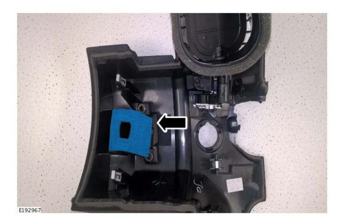
3. NOTE: The interior temperature sensor insulator foam must cover the edge around the duct ( / ).
