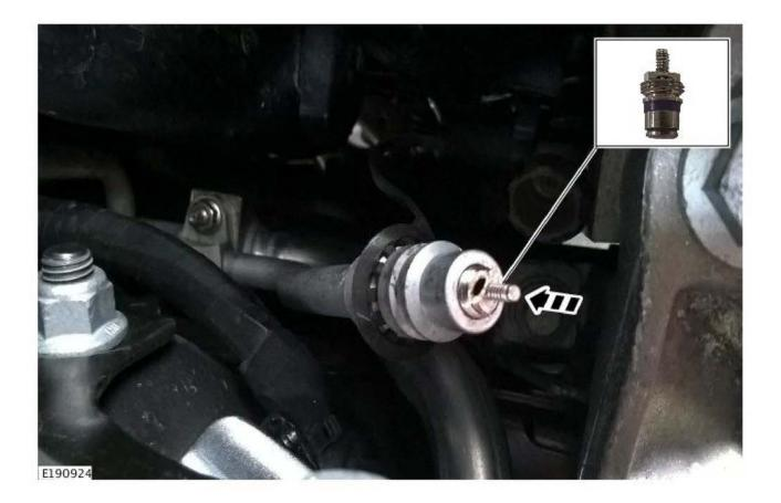
Charge the Air Conditioning system (see TOPIx Workshop Manual section 412-00: General Procedures - Air Conditioning (A/C) System Recovery, Evacuation and Charging GTDi 2.0L Petrol/GTDi 2.0L Petrol - SULEV).
