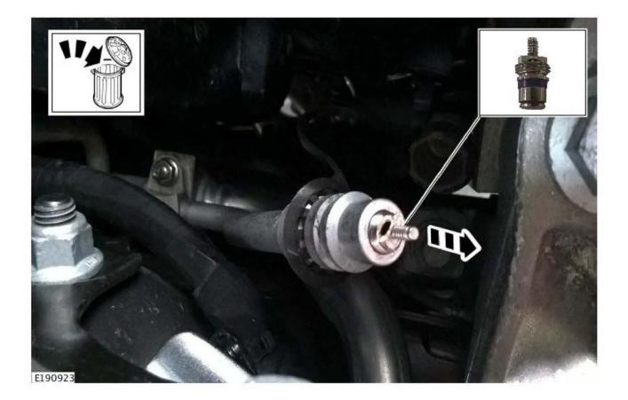
3. ONOTE: Repeat this step on both Air Conditioning charge port Schrader valves. Using a suitable tool, install a new Air Conditioning (A/C) charge port Schrader valves (turn clockwise).
