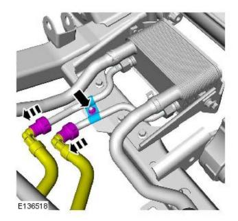
5. ONOTE: Use a suitable container to catch any transmission fluid spillage.
